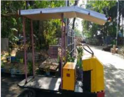
As a trial measure 180 Wp Solar Photo Voltaic panel installed in one Platform Truck for charging the battery when it is on use.
